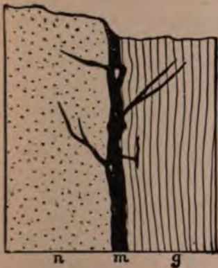
FIG 14 a .—SECTION OF A PYRITE VEIN OF ERTELI MINE NO. 1. (Vogt.) n , NORITE; g , GNEISS; m , PYRITE MASS. HIGHT OF SECTION, 5 METERS
